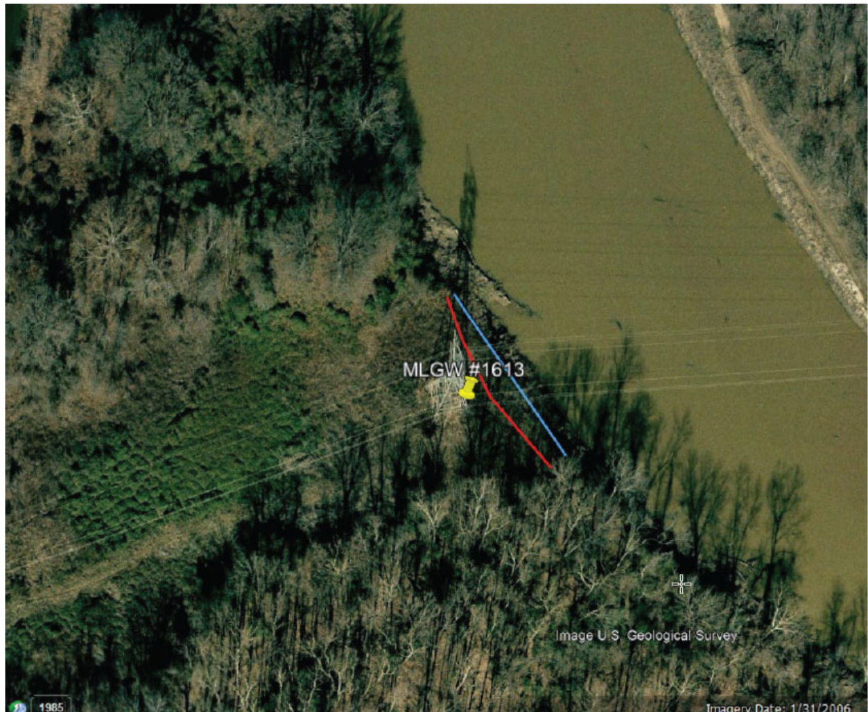
Figure 3. Wolf River Top Bank Comparison at Tower #1613 between 31 January 2005 (blue) and 05 September 2021 (red).
